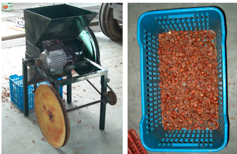
Figure 3- Shell equipment AGRO 162 and shelled hazelnuts
