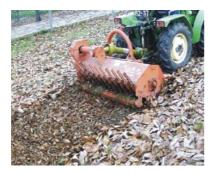
Figure 1- Crushing equipment with hammers
