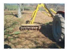
Figure 2- Crushing equipment with knifes
