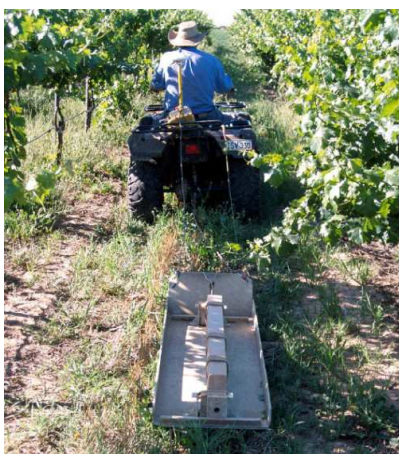
Figure 27: EM38 pulled behind a four-wheel motorbike (source: Bramley, CSIRO).
