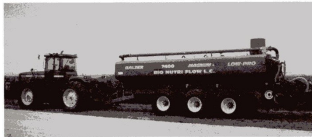
Illustration of a manure applicator equipped to provide map-based control of the application process
