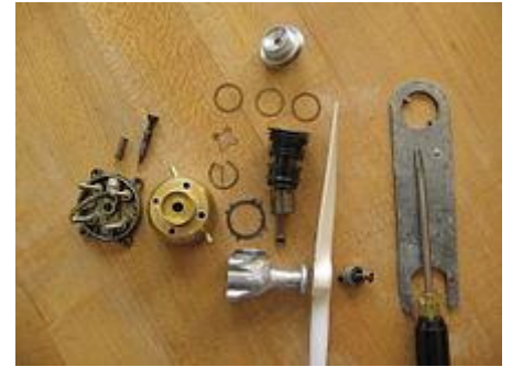
A Cox Babe Bee 0.049 cubic inch (0.8 cubic cm) reed valve engine, disassembled, uses glow plug ignition. The mass is 64 grams.
