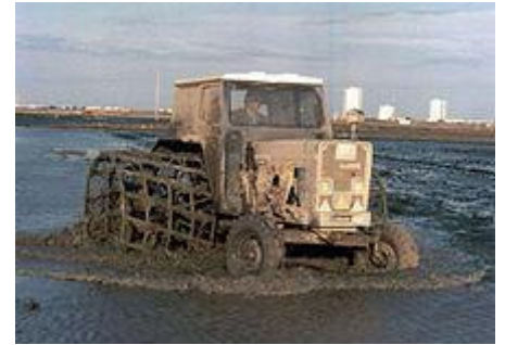
Ebro farm tractor with steel wheel extensions. This arrangement is often used in muddy conditions that are found in paddy farming of rice.
