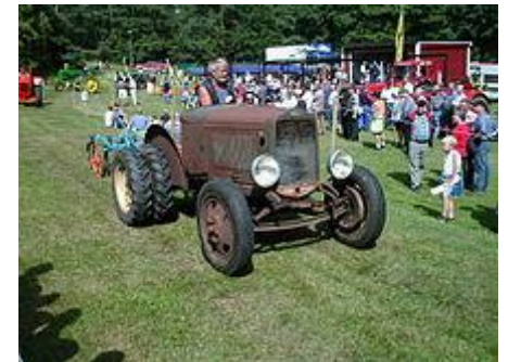
A Ford rebuilt to an EPA tractor
