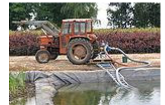
A farm tractor used to power a pump for irrigating a plot of land
