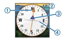
The course pointer ① indicates your relationship to the course line leading to the destination. The course deviation indicator (CDI) ③ provides the indication of drift (right or left) from the course. The scale ② refers to the distance between dots ④ on the course deviation indicator, which tell you how far off course you are.
