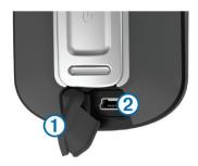
2 Plug the small end of the USB cable into the mini-USB port.
