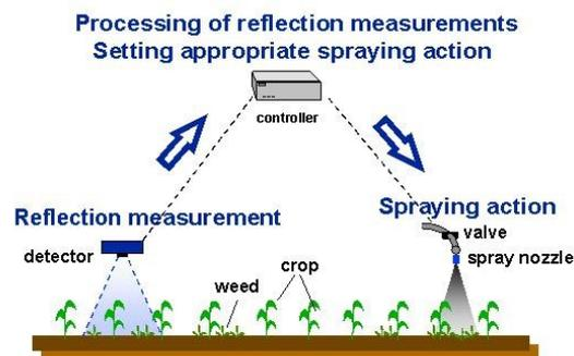
Figure 3 - Optical weeds detection for herbicides application in real time.
