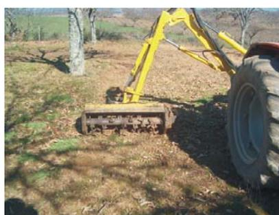
**Figure 2-** Crushing equipment with knives
