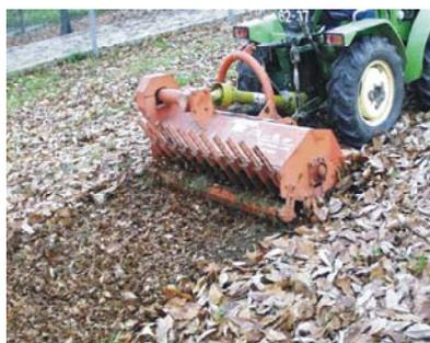
**Figure 1-** Crushing equipment with hammers
